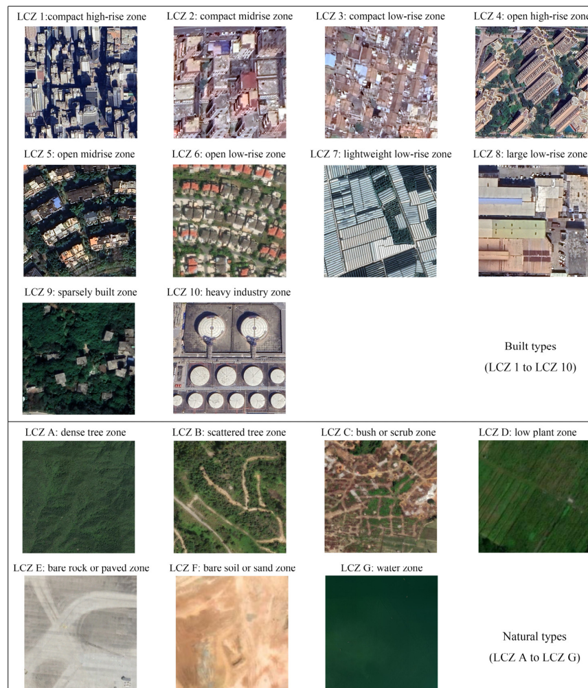
Figure A1. Examples of representative LCZs from Guangdong–Hong Kong–Macao Greater Bay Area Central (GBAC) region. This classification system is segmented into built types (LCZ 1 to LCZ 10) and natural types (LCZ A to LCZ G).
